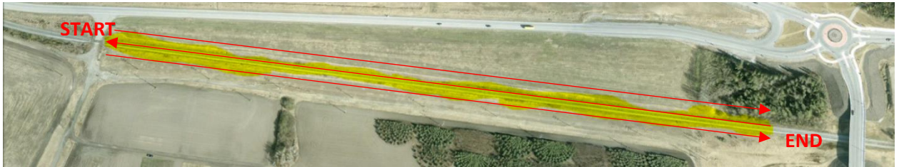
Figure 4. Sample of linear flight pattern over road segment. 75% frontal overlap and 75% side overlap is recommended change detection/linear orthomosaic operations. Segment stitching requires an additional 100' of overlap between segment ends.
