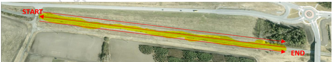
Figure 4. Sample of linear flight pattern over road segment. 75% frontal overlap and 75% side overlap is recommended change detection/linear orthomosaic operations. Segment stitching requires an additional 100' of overlap between segment ends.
